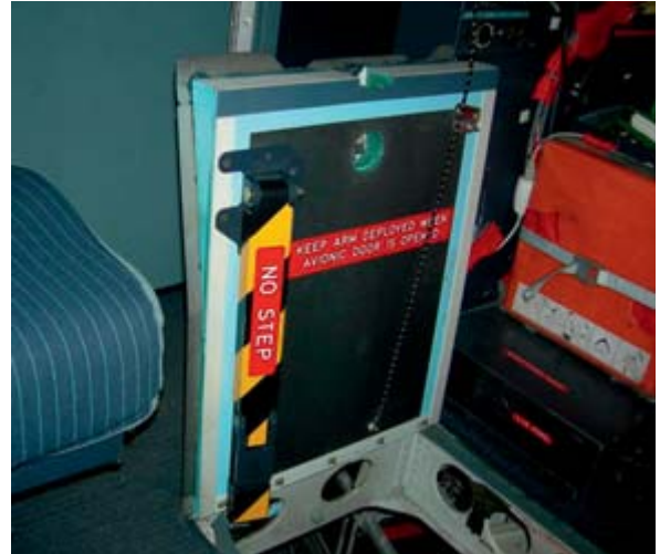
Figure 3: Avionics access hatch with folded protective arm
