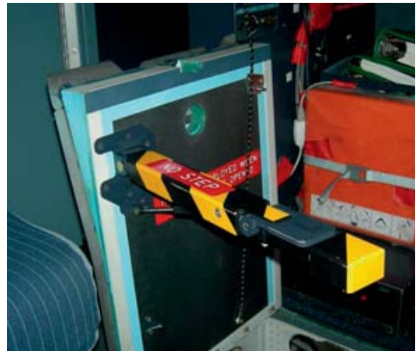
Figure 4: Avionics access hatch with unfolded protective arm
